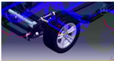
3D MBS suspension / tire clearance analysis
